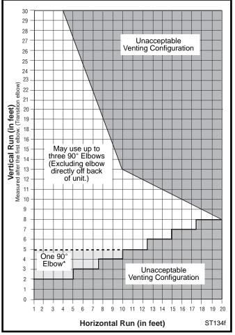
Fig. 7 Horizontal vent termination window.
